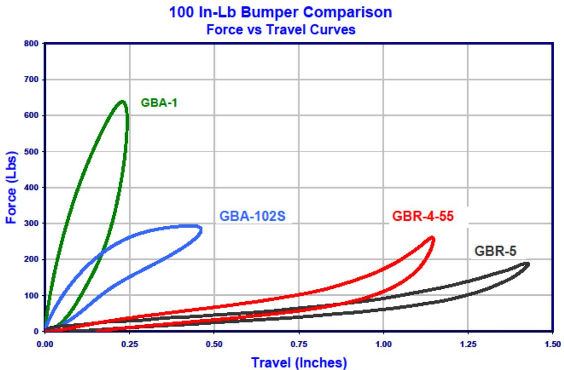
As can be seen, all four bumpers are rated at a similar energy, but have significantly different performance curves. If there is limited space and end force is not critical, the GBA-1 might be the best choice. If longer travel with a softer initial spring rate and lower end force is important, the GBR-4-55 or GBR-5 would be a better selection. Finally, a compromise between all of the considerations would be the GBA-102S which is midrange in both travel and end force.
